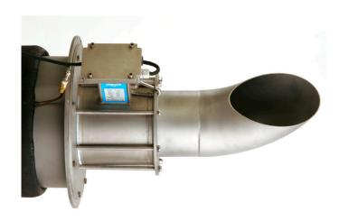
The SEWER-MAG<sup>TM</sup> is an insertable full bore electromagnetic flow meter sensor. It ensures extremely accurate flow determination even under difficult flow conditions. The SEWER-MAG<sup>TM</sup> is usually temporarily installed in sewer networks to verify or calibrate existing flow meters.
