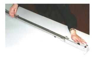
To calculate the crimp in yarn affected by knitting or weaving, to determine actual yarn usage. Threads are removed from a strip of fabrics of known length, straightened by a tension, then measured in the straightened state. Two tension ranges available (0-35 g and 0-175 g) and test length is 120 cm (48 inches).
