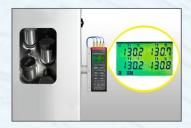
Temperature difference among dyepots within 1°C (Measuring by thermal instrument)
