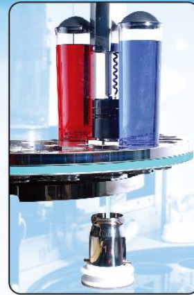
無管路滴液實況，精確滴液 Tubeless dispensing, high accuracy
