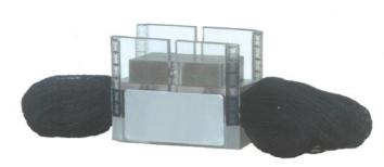
Simple device to define the volume occupied at a given pressure by the mass of a specified amount of the yarn. Unit of bulk = cm<sup>3</sup>/g. The apparatus consists of a channel with graduated scales on each corner in which a skein is placed containing a known number of ends. A load of 500 g is applied to produce a pressure of 10 g per cm<sup>2</sup>.
